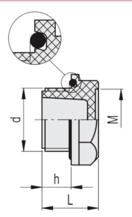
$\begin{array}{lll} d & = M \ 27x1.5 \\ D & = 37 \\ h & = 12 \\ L & = 22 \\ M & = 25 \\ s & = 32 \\ Weight \ (g) = 14 \end{array}$
